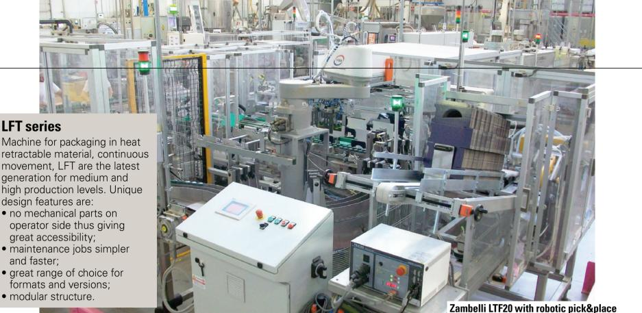
total accessibility, operation with no resistance and can be immediately reset in case of an E-stop.
